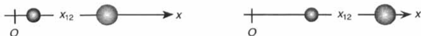
FIGURE 1.1 If two particles interact through a mutual potential depending only on their separation x_{12} , independent of the choice of origin O , then the total momentum is conserved.
