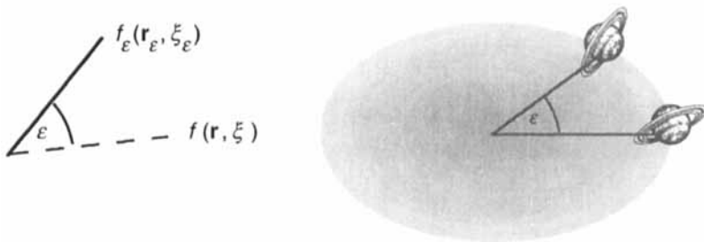
FIGURE 3.12 The difference between total angular momentum and orbital angular momentum is demonstrated by the differing effects of rotation through a small angle \epsilon of a function f describing a system that has some internal degrees of freedom, such as the rings around a planet. The planet orbital angular momentum will have \ell > 0 if the orbit is elliptical, as shown.
