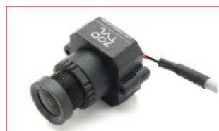
FatShark 700TVL CMOS camera provides excellent short range video.
