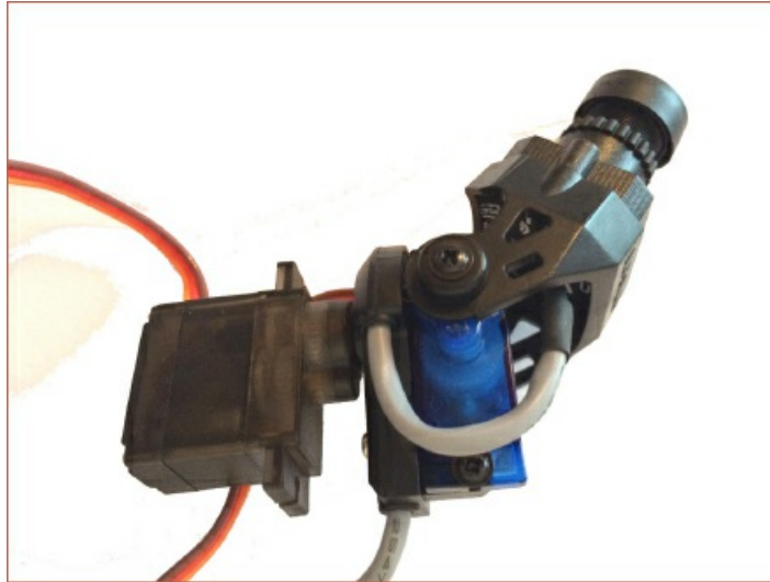
A simple camera gimbal setup providing both pan and tilt.
