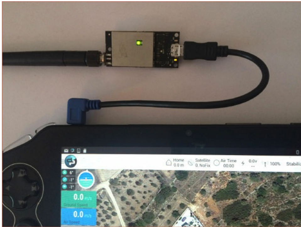
OTG USB cable used to attach telemetry to Nexus 7.
