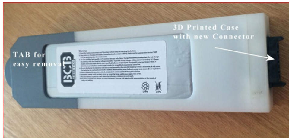
Battery case 3D printed with plug-in female connector.
