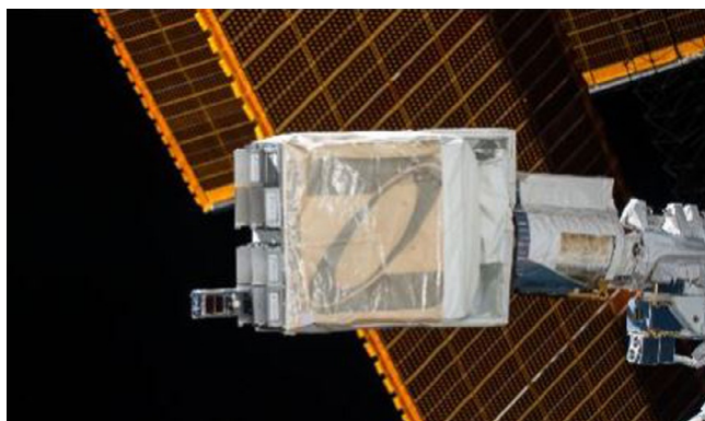
Fig. 2 Nanoracks ISS CubeSat deployer. Courtesy Nanoracks.
