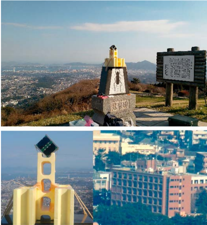
Fig. 5 Photograph of open-air long distance communication test. Actual setup at the mountain (top), closer view of satellite (bottom left) and view of ground station from the mountain (bottom right).
