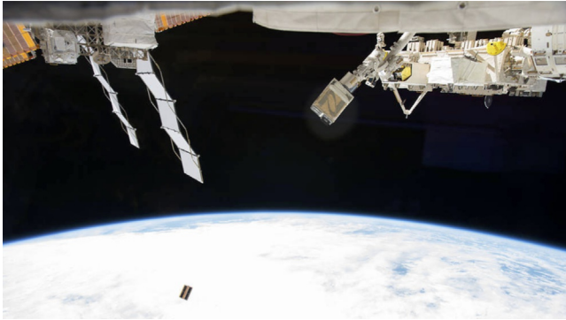
Fig. 4 Photograph of the 6U, 11-kg EcAMSat nanosatellite ( lower left-center ) above Earth seconds after deployment from the ISS (deployer is at mid-upper center of photo). It was the first 6U biology satellite and the first biological science satellite of any size to be deployed from ISS. Credit: NASA.
