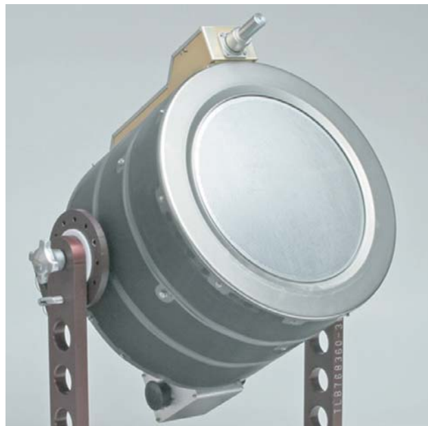
Fig. 9-4. Photograph of the 25-cm XIPS ion thruster (photo courtesy of L-3 Communications, Electron Technologies, Inc.).
