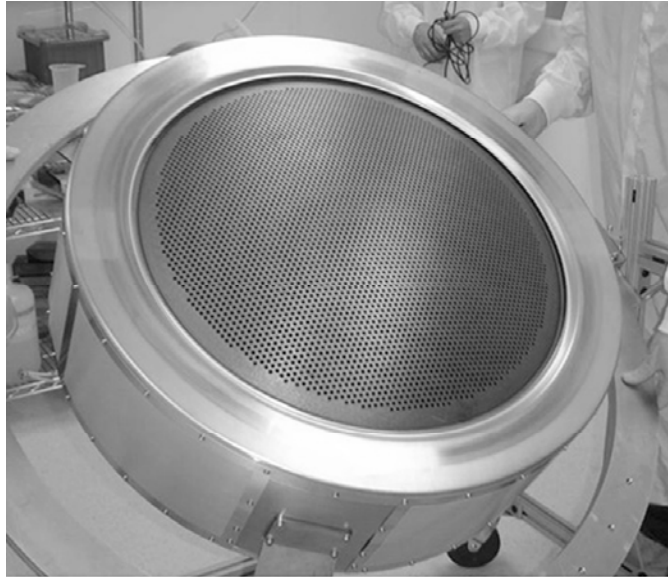
Fig. 1-2. Photograph of the NEXIS ion thruster [27] showing the 57-cm-diameter multiaperture grids and plasma screen enclosing the thruster body.
