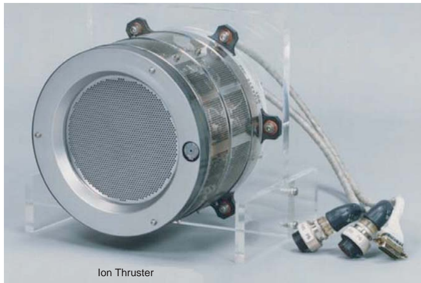
Figure 9-8. Photograph of the ETS-8 Kaufman ion thruster (from [23]).
