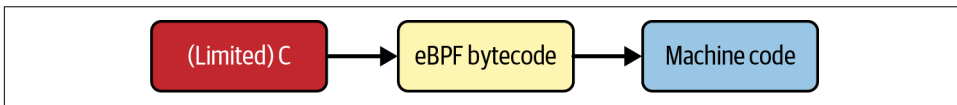
Figure 3-1. C (or Rust) source code is compiled into eBPF bytecode, which is either JIT-compiled or interpreted into native machine code instructions
