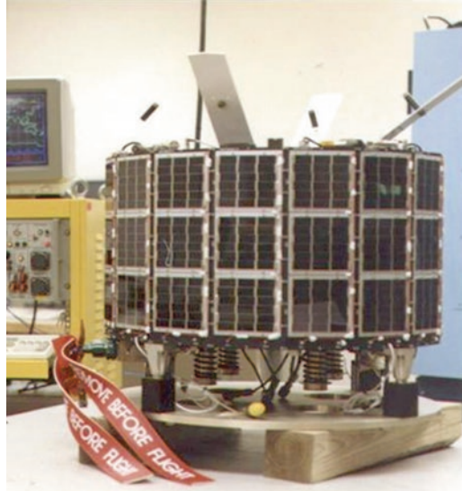
Fig. 2.2 180 lbs, 89.5^\circ , 756 \times 887 km orbit, gravity gradient stabilized communications satellite
