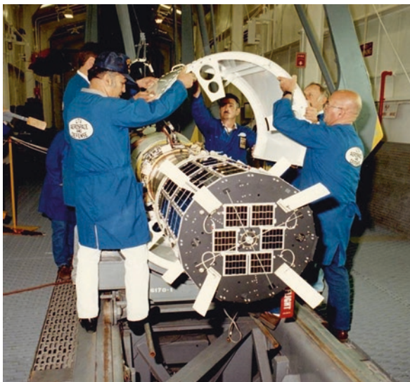
Fig. 2.3 Two 170-lbs polar orbit digital store-forward communications satellites
