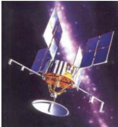
Fig. 2.5 400 lbs, 822 km Polar orbit, 3-axis pitch bias momentum stabilized satellite. Gimbaleddish antenna & deployable solar panels
