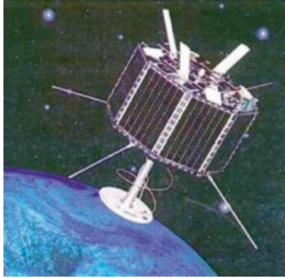
Fig. 2.4 190 lbs Polar orbit, 800 km altitude radar calibration satellite with 17 deployable antennas
