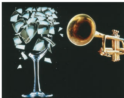
FIGURE 11–19 This goblet breaks as it vibrates in resonance to a trumpet call.
