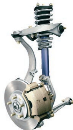
FIGURE 11-4 Photo of a car's spring. (Also visible is the shock absorber, in blue—see Section 11-5.)
