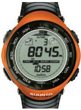
FIGURE 24-52 Watch-face LCD display with altimeter. The black segments or pixels have a voltage applied to them. Note that the 8 uses all seven segments (pixels); other numbers use fewer.
