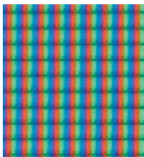
FIGURE 24-53 Arrangement of subpixels on a TV or computer display (enlarged).
