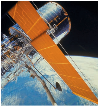
FIGURE 25–32 Hubble Space Telescope, with Earth in the background. The flat orange panels are solar cells that collect energy from the Sun to power the equipment.
