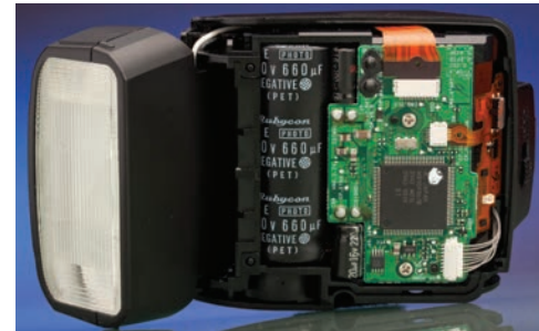
FIGURE 17-20 A camera flash unit. The 660- \mu\text{F} capacitor is the black cylinder.
