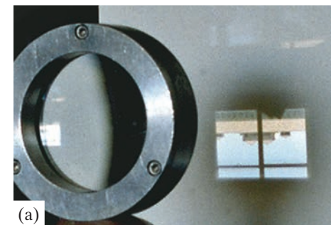
FIGURE 23-38 (a) A converging lens can form a real image (here of a distant building, upside down) on a white wall. (b) That same real image is also directly visible to the eye. [Figure 23-31d shows images (graph paper) seen by the eye made by both diverging and converging lenses.]
