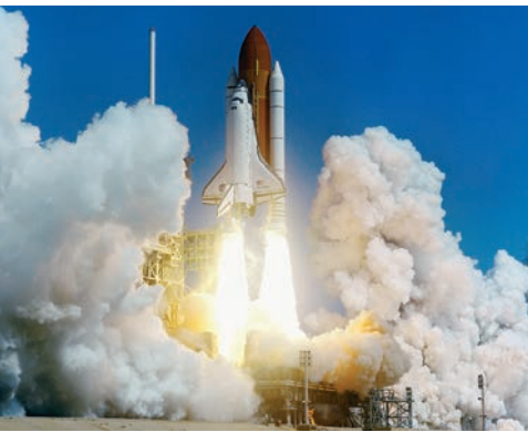
FIGURE 4–10 Another example of Newton’s third law: the launch of a rocket. The rocket engine pushes the gases downward, and the gases exert an equal and opposite force upward on the rocket, accelerating it upward. (A rocket does not accelerate as a result of its expelled gases pushing against the ground.)
