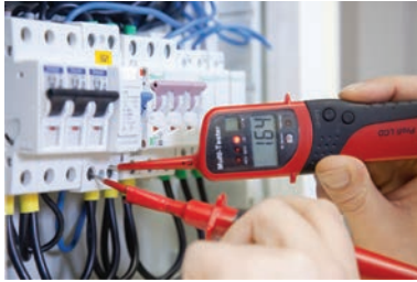
FIGURE 19–30 (a) An analog multimeter. (b) An electronic digital meter measuring voltage at a circuit breaker.
