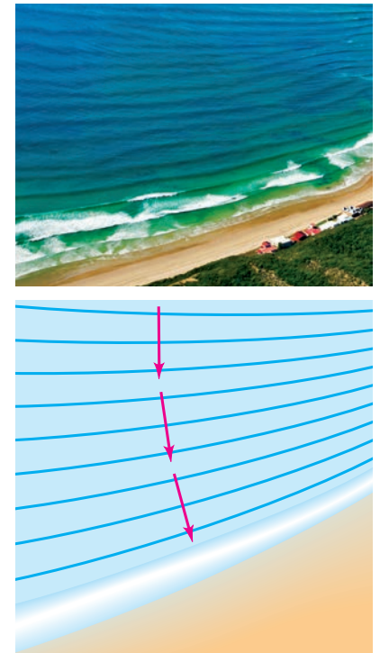
FIGURE 11-43 Water waves refract gradually as they approach the shore, as their velocity decreases. There is no distinct boundary, as in Fig. 11-42, because the wave velocity changes gradually.
