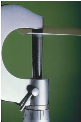
FIGURE 1-11 Example 1-7. Micrometer used for measuring small thicknesses.
