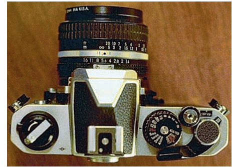
FIGURE 25–5 On this camera, the f -stops and the focusing ring are on the camera lens. Shutter speeds are selected on the small wheel on top of the camera body.
