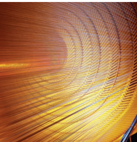
FIGURE 30–16 Multiwire chamber inside the Collider Detector at Fermilab (CDF). Figure 32–15 in Chapter 32 was made with this detector.
