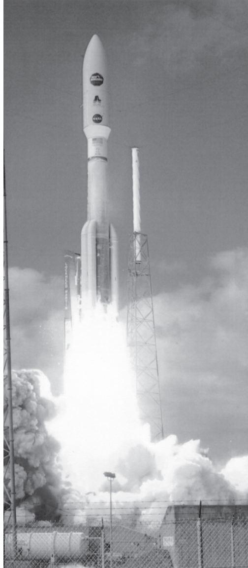
Figure 1-13 Atlas V space launch vehicle with three (or five) strap-on stages using Aerojet solid rocket motors and a central Energomash (Russia) RD-180 liquid propellant booster rocket engine running on LOX/kerosene. See Table 1-3 for key parameters.
