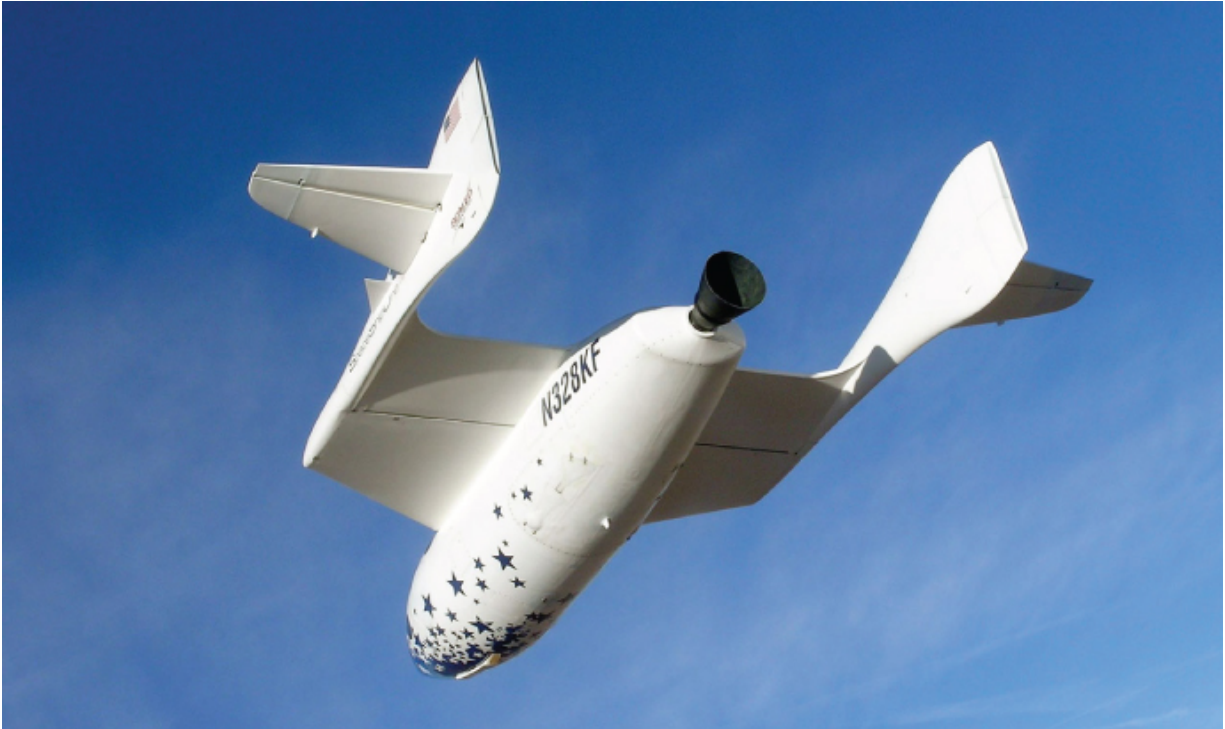
Figure 16-3 SpaceShipOne gliding down for landing. This air ship uses a hybrid propulsion system to produce its main thrust. The propellant is N_2O -HTPB.
