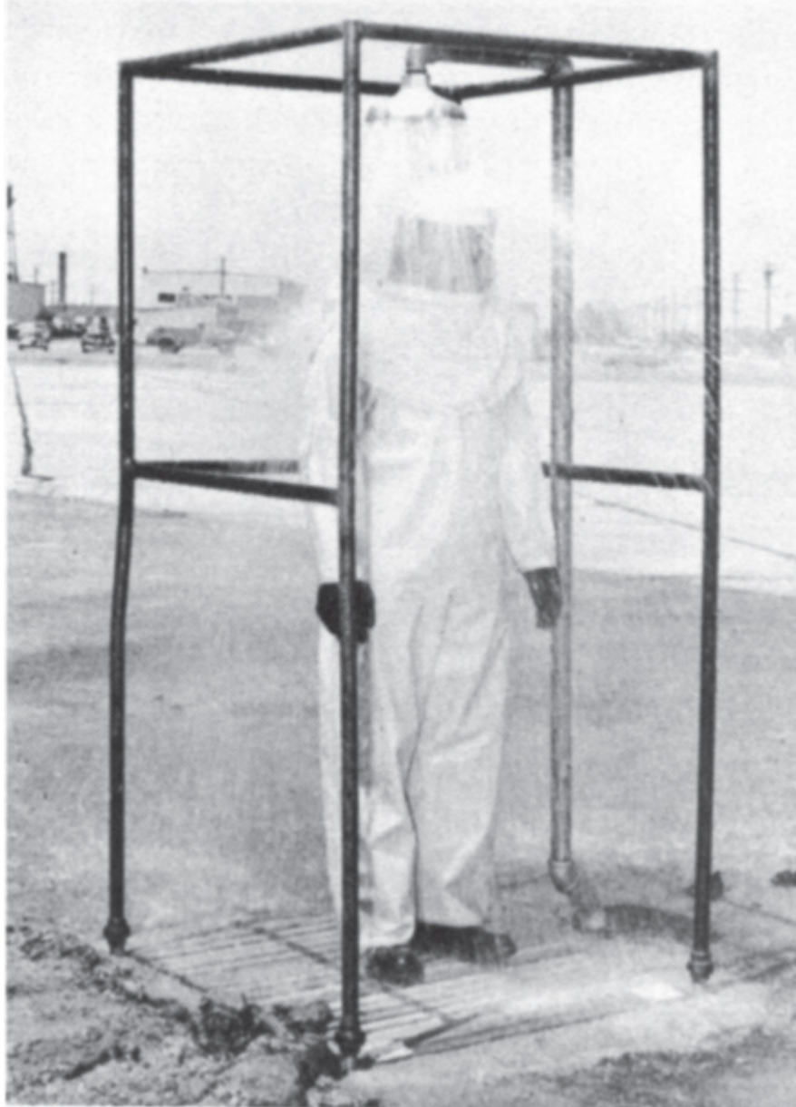
Figure 21–4 Plastic safety suit, gloves, boots, and hood used by test personnel in handling hazardous and/or corrosive liquid propellants. The safety shower, which starts automatically when a person steps onto the platform, washes away splashed or spilled propellant.
