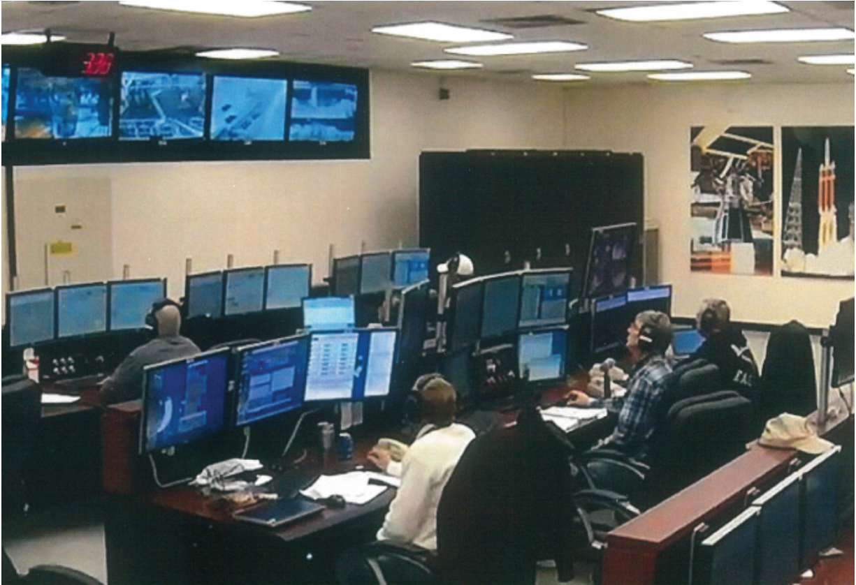
Figure 21–3 Photograph of an actual RS-68A acceptance test. The test conductor is in the middle back row; to his right is the engine test article engineer and to his left is the controls and vehicle simulation engineer (the row in front primarily controls facility stations, like the oxygen and hydrogen systems). Up on the top are units monitoring engine firing. Present day testing is nearly all controlled remotely with computers, which also display read-out meters and act as data recorders.
