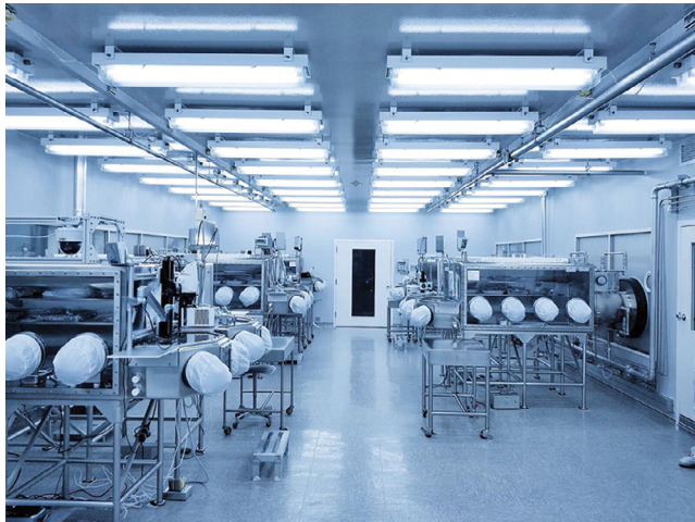
Fig. 11.2 Apollo samples are handled in gloveboxes under high-purity gaseous nitrogen in the Pristine Sample Laboratory. Each stainless steel glovebox is dedicated to a specific Apollo mission to avoid cross-contamination. (Credits: A. Hutzler).
