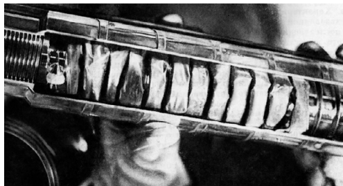
Fig. 3.25 Reception drum with a flexible sampler. With the permission of the Vernadsky Institute.
