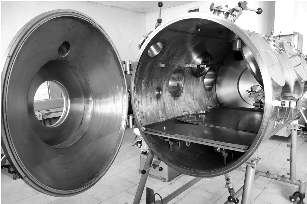
Fig. 3.31 A hinged lid of the receiving lunar chamber. (Photo by the author. With the permission of the Vernadsky Institute).
