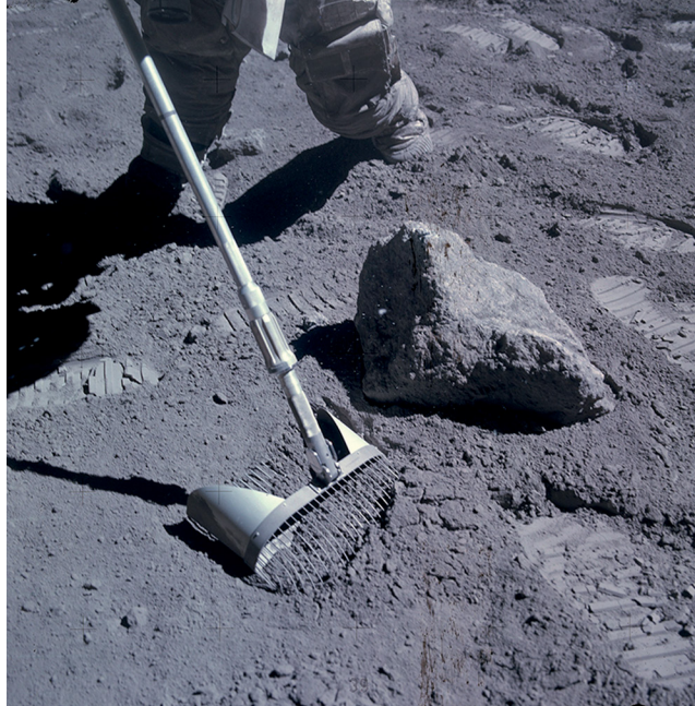
Fig. 2.2 Lunar rake used to separate rocks from the surface regolith. (NASA photograph AS16-116-18690).
