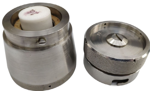
Fig. 3.36 A sealed stainless steel container for storing and transporting samples of lunar soil. Sizes: height is 80 mm, a cover diameter is 60 mm, and a bottom diameter is 70 mm. Mass is 1452 g. (Photo by the author. With the permission of the Vernadsky Institute).
