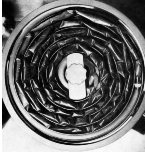
Fig. 3.39 An elastic sampler with lunar soil in a spiral groove. (With the permission of the Vernadsky Institute).
