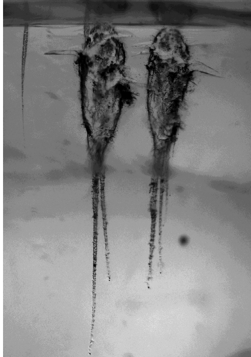
Fig. 4.6 Cometary particles impacting Stardust aerogel collector tiles created several types of tracks. Single, strong particles created long, thin carrot tracks like the one on the left of the image. Weaker aggregate particles came apart during impact and produced more bulbous tracks like the two in the center of the image. Particles in this image entered from above and the surface of the aerogel is at the top of the image.
