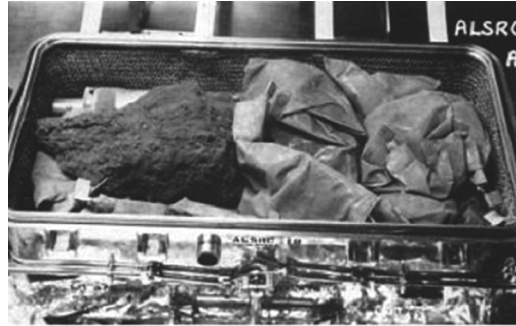
Fig. 15.2 Apollo 16 LSRC upon opening in the Lunar Receiving Laboratory with a large rock inside (Credits: NASA, 372–36,984 photo).
