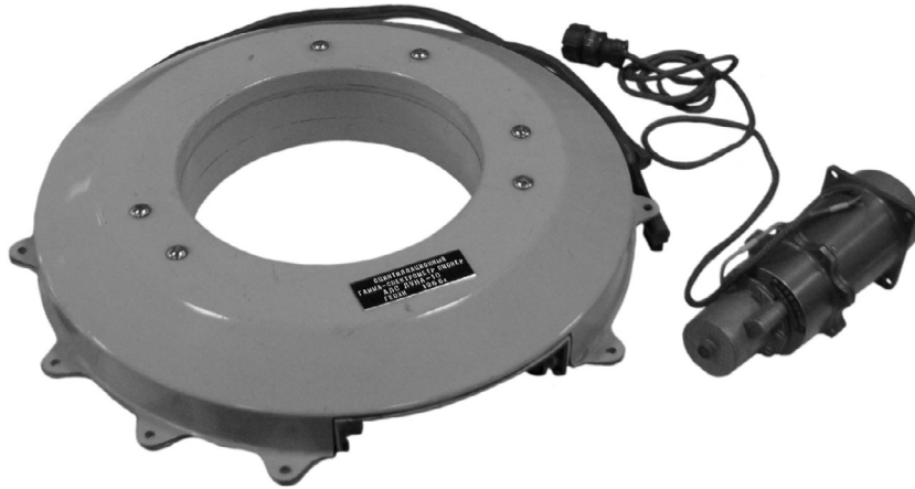
Fig. 3.14 General view of the gamma spectrometer for the Luna-10 spacecraft. (Photo by the author. With the permission of the Vernadsky Institute).
