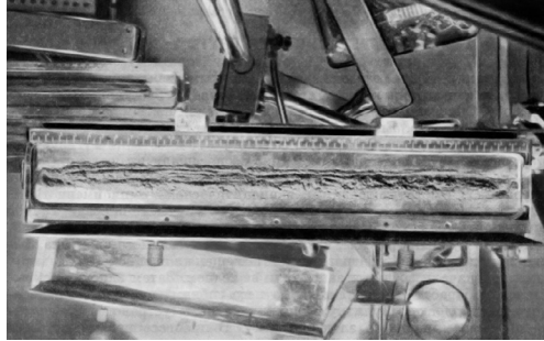
Fig. 3.41 A sample of lunar soil delivered by Luna-24 on one of the seven trays in the receiving lunar chamber. (With the permission of the Vernadsky Institute).
