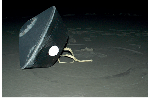
Fig. 4.5 The Stardust Sample Return Capsule as found during its recovery from the Utah Test and Training Range.
