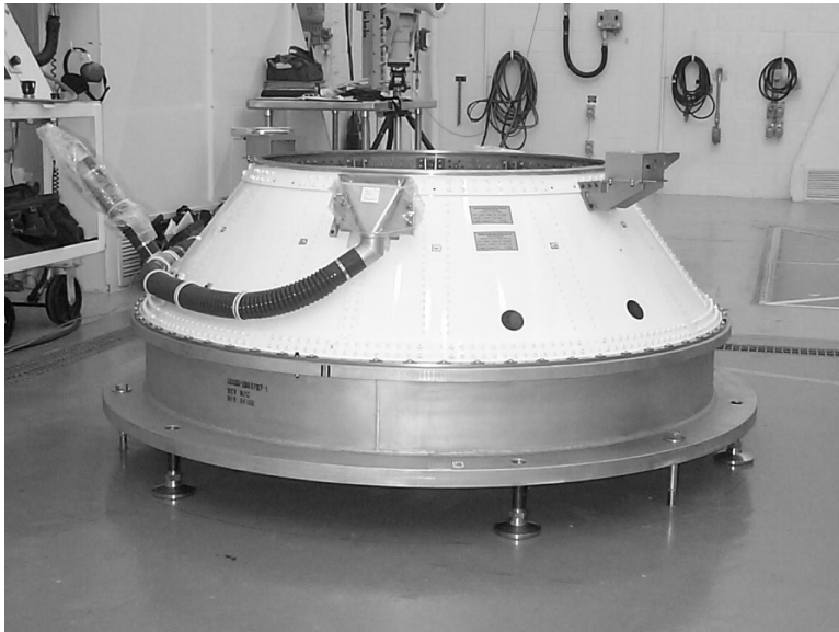
Figure 8.3 Launch vehicle to spacecraft adaptor. (Reproduced by permission of EADS Astrium Ltd.)
