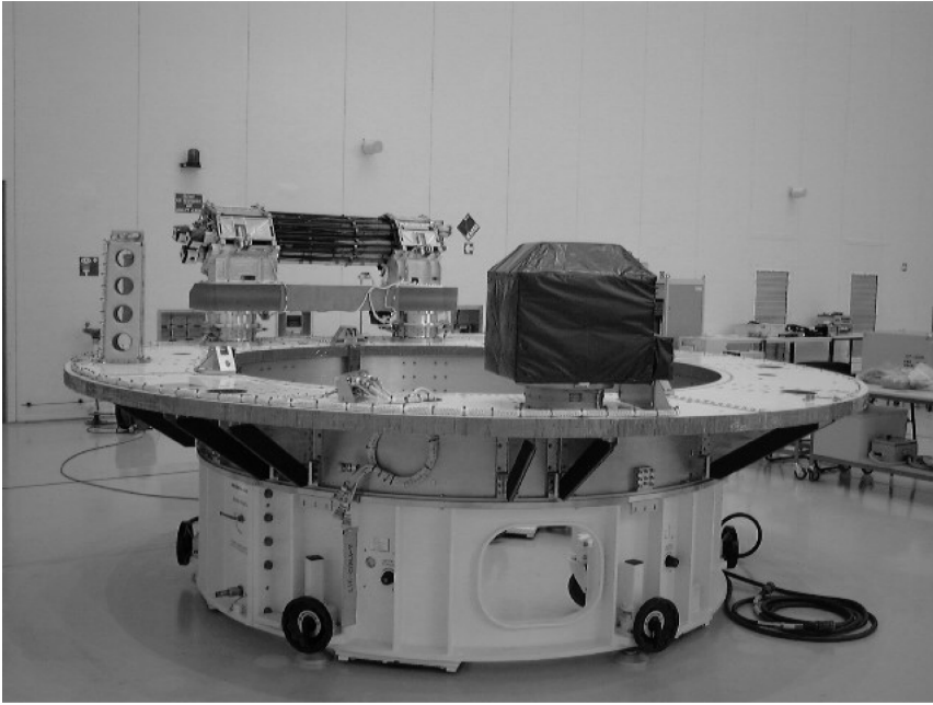
Figure 8.2 Ariane Structure for Auxiliary Payloads (ASAP5) for Ariane 5. (Reproduced by permission of EADS Astrium Ltd.)
