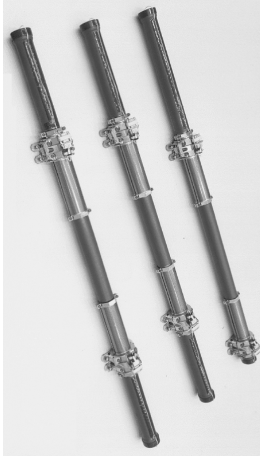
Figure 9.8 Magnetic torquers. The three torque rods shown are those used on the EURECA spacecraft, and are each in excess of a metre in length. (Reproduced by permission of Dutch Space BV)
