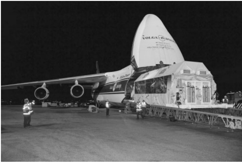
Figure 17.12 Shipment to the launch site: Herschel, in its container, is loaded into an Antonov transport aircraft. Note container air conditioners, and the bank of gas bottles for purging the interior. (Photo: ESA, Anneke Le Floc'h)
