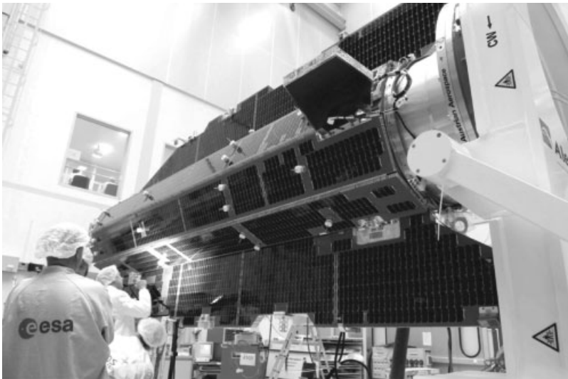
Figure 17.9 GOCE (Gravity field and steady-state Ocean Circulation Explorer) spacecraft attached to its Integration and Turn-over Stand for detailed inspection of solar cells. (Photo: ESA, Anneke Le Floc’h)
