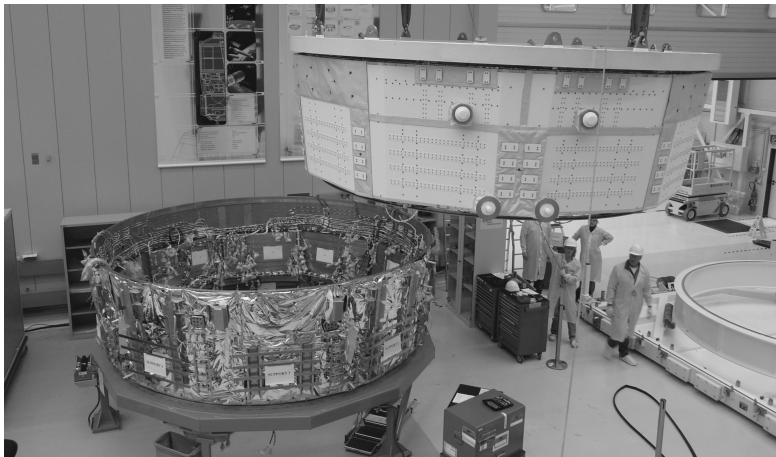
Figure 11.14 VCHPs integrated in the ATV avionics bay radiators — lower left, during integration and, upper right, a completed avionics bay. (Reproduced by permission of EADS Astrium)
